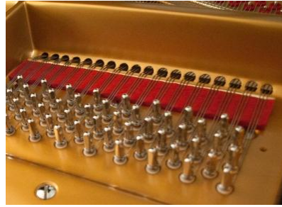
Fig.: A sound reflecting rim, a strictly limited soundboard and pressure bar bridges.
